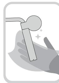
Wipe steam wand & tip with a damp cloth. Remove the wand cover to fully clean the steam wand.
