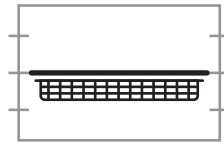
Baking pan in guide rails below wire rack
