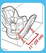
Lower anchor attachment can only be used if the vehicle lower anchor spacing is 11" (28 cm) from the center of one lower anchor to the center of the other lower anchor.
