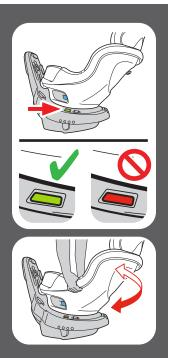
Check the turn lock indicator on the side of the base. If the indicator is red, the seat is NOT securely locked in place. The seat is securely locked in position when the indicator is green.
